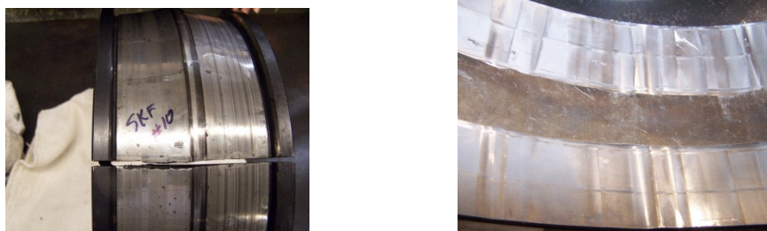
Figure 21. Failed Inner and Outer Bearing Races
