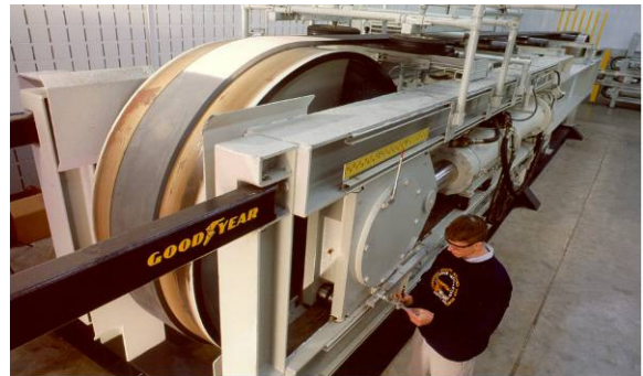
Figure 12. 2-Pulley Dynamic Splice test machine
