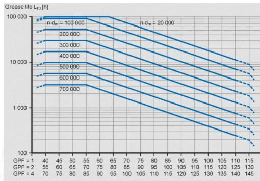
Operating temperature [°C] for various grease performance factors (GPF)
