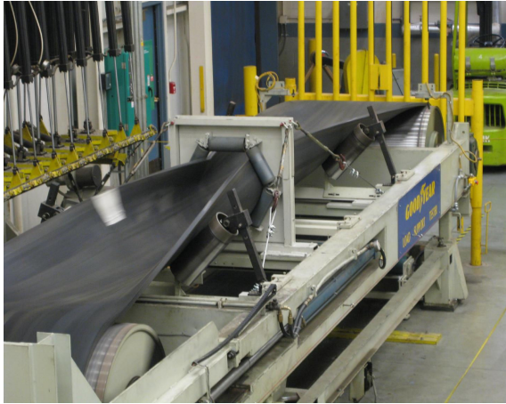
Figure 3. Pipe belt transition test
