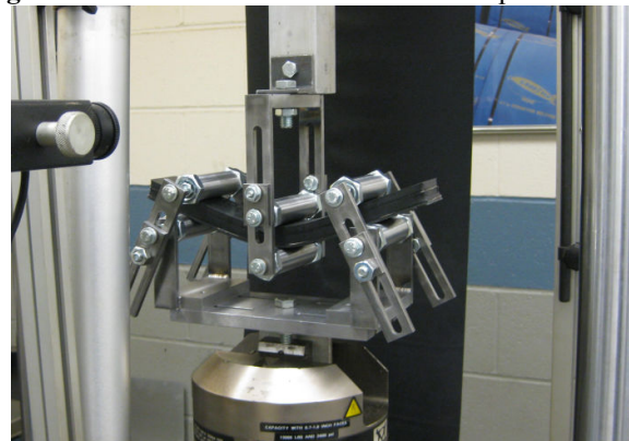
Figure 2. 3 point bending stiffness test
