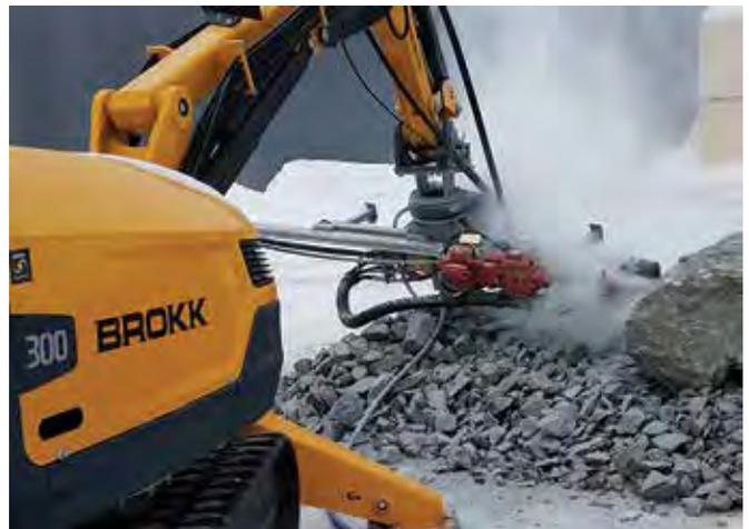
The MMB326 hydraulic drifter rock drill attachment.
