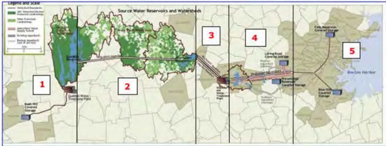
water was conveyed by the Wachusett/Weston Aqueduct to the Weston Reservoir and then by pipeline to the Chestnut Hill and Spot Pond Reservoirs. Work was completed in 1905 and the reservoir first filled in May 1908. The Wachusett system was built to service the 29 municipalities within a 16-km (10-mile) radius of the Massachusetts State House. At the time, the Wachusett Reservoir was the largest public water supply reservoir in the world with a capacity of 246 GL (65 billion gal).
