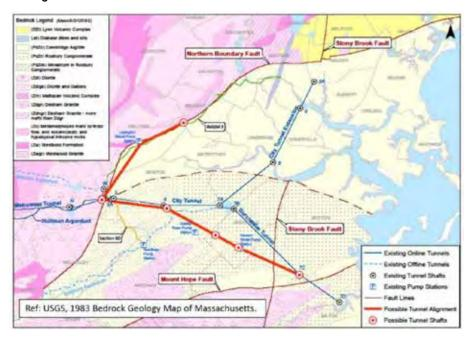
The quality of rock encountered along the City Tunnel is noted by Tierney as being excellent for tunneling. Just 5 m (16 ft) of the 7.7-km (4.78-mile) tunnel required structural steel support with the remaining approximately 7.7 km (4.7 miles) of tunnel mined with no need for temporary supports. The bedrock through which the City Tunnel extends was considered unusually good as compared to that encountered along other tunnels previously mined through similar geology in the greater Boston area.
