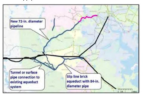
Given the difficulties associated with the construction and significant community impacts associated with large-diameter surface pipe together with operational reliability concerns, MWRA staff are pursuing a preferred all-tunnel redundancy alternative. The preliminary alignment, which will be subject to more detailed review and alternatives analysis during the public review period, is shown in Fig. 8.
