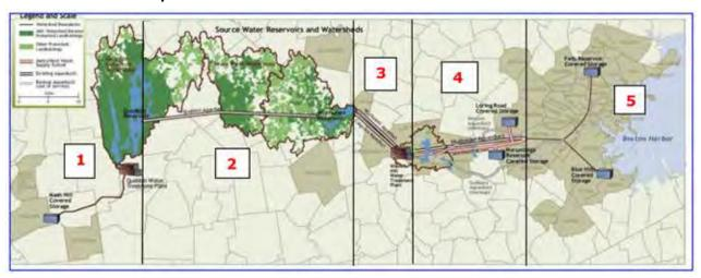
water was conveyed by the Wachusett/Weston Aqueduct to the Weston Reservoir and then by pipeline to the Chestnut Hill and Spot Pond Reservoirs. Work was completed in 1905 and the reservoir first filled in May 1908. The Wachusett system was built to service the 29 municipalities within a 16-km (10-mile) radius of the Massachusetts State House. At the time, the Wachusett Reservoir was the largest public water supply reservoir in the world with a capacity of 246 GL (65 billion gal).
