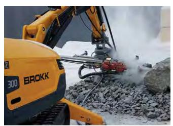
The MMB326 hydraulic drifter rock drill attachment.
