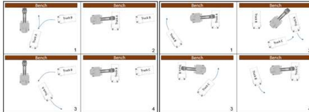
Figure 4-8 Single-side method (left) and double-side method (right)
