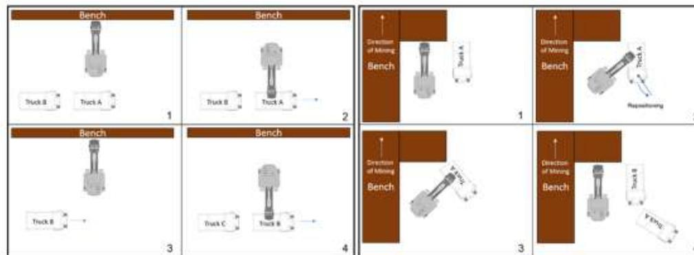
Figure 4-9 Drive-by method (left) and modified drive-by method (right)
