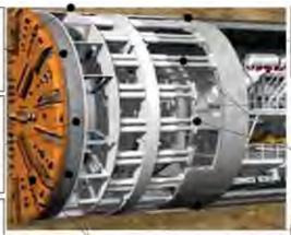
Ground conditioning optimization: Apply the optimal combination of conditioning types - including water, bentonite, foam, and polymers - and their individual recipes to achieve the desired outcomes, e.g., minimize wear, clogging risk, cost; maximize muck flowability through cutterhead, chamber and screw conveyor, etc. Annulus grouting: inject annulus grout around liner with requisite pressure to completely fill annulus gap with the theoretical volume.
