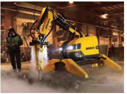
The Atomized Water Mist System requires less water than other methods, just 0.2 L/ min (6.76 oz per minute).
