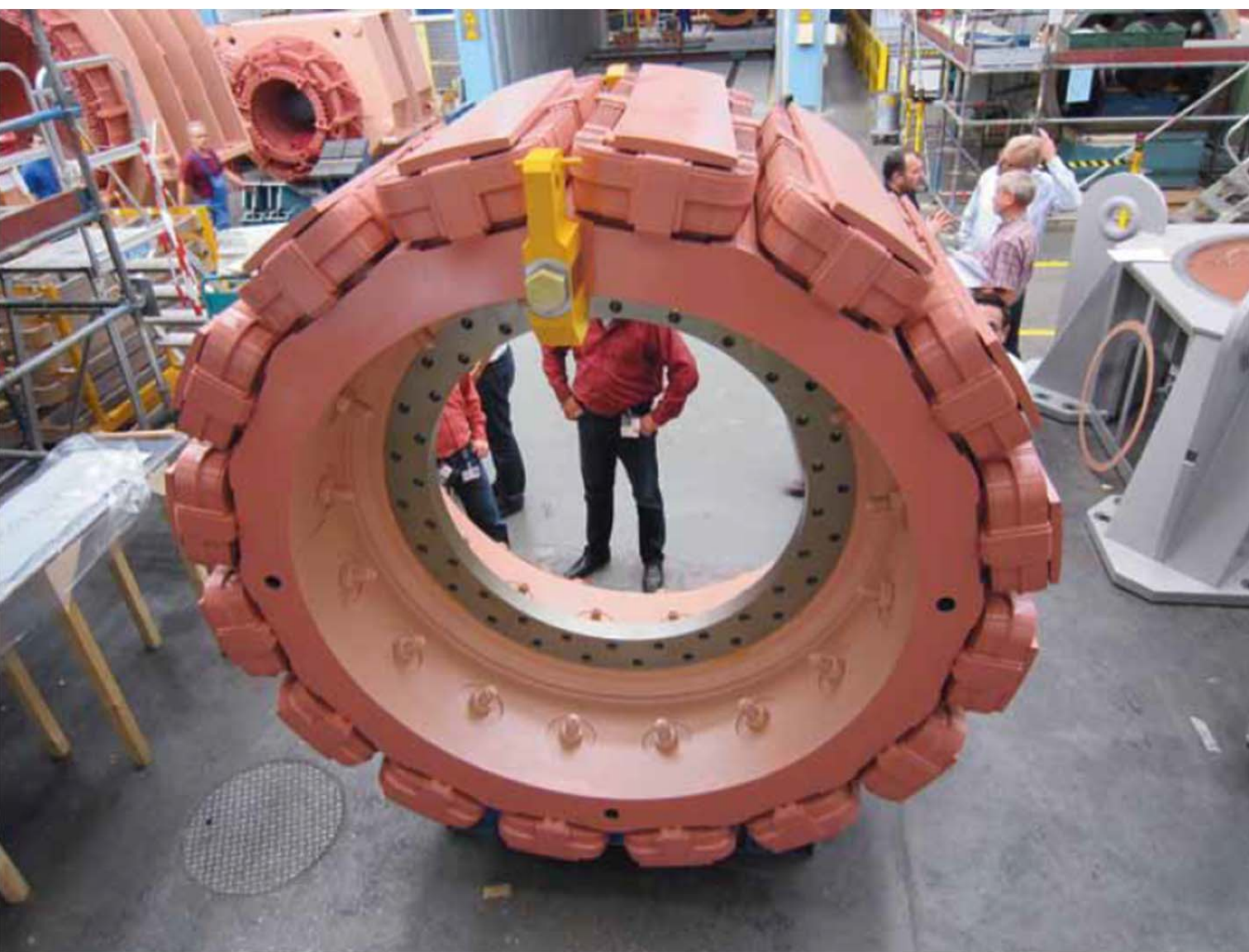
Figure 1: Gearless Drive rotor during shop inspection at Siemens
