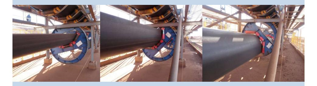
Most troughed turnover has support and guide rolls inside, contacting the dirty side. But there are also designs with support rolls on outside bottom cover.
