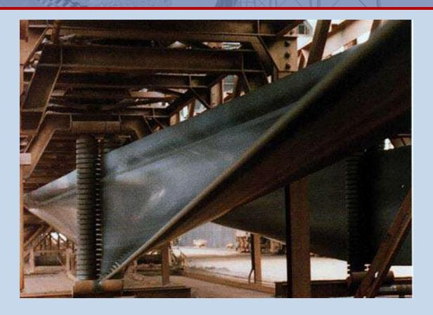
• Poorly designed (mostly being too short) flat turnover can have very high edge stress, compressive center stress, and a buckled shape.
