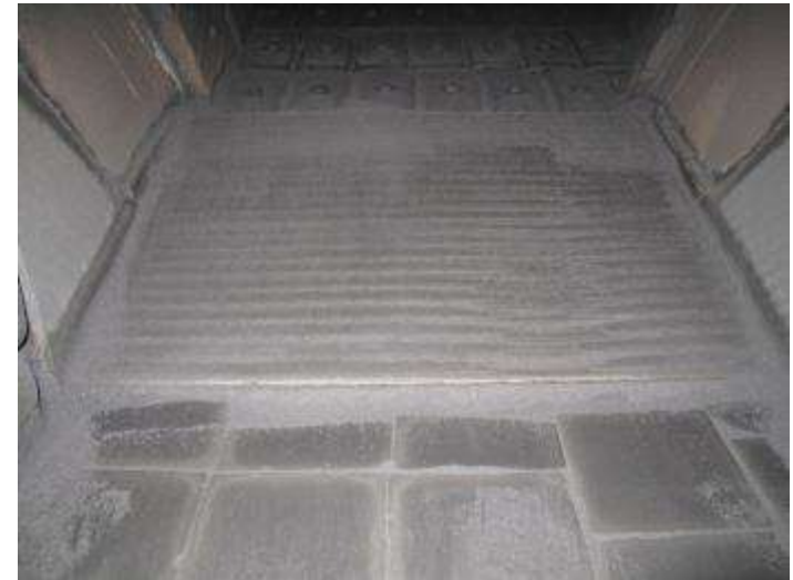
Transfer chute for cooking coal after 12 month in operation VAUTID-143 wear plates 3/8" on 3/8" (10+10mm)
