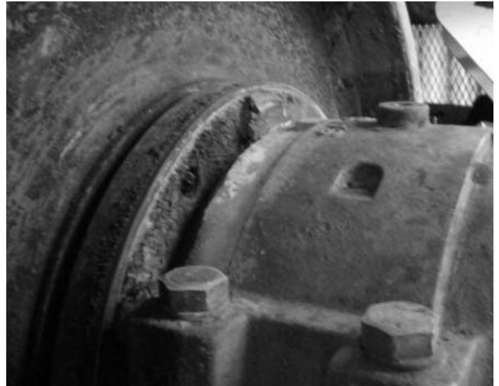
Figure 5 – Example of a Pulley that has “walked” on the shaft.
