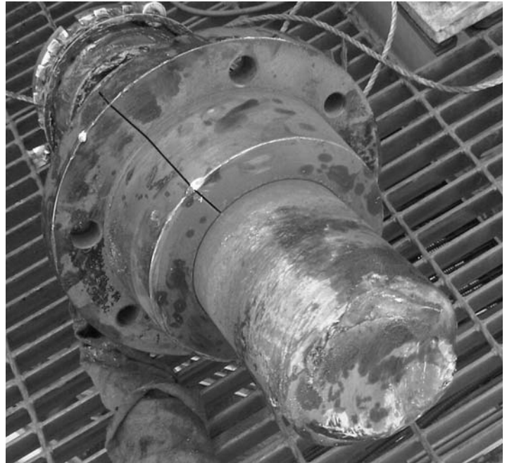
Figure 12 – Shaft Failure at 380% of Design Load
