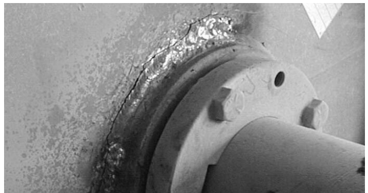
Figure 3 – Example of Re-Weld Failure at the Hub Weld
