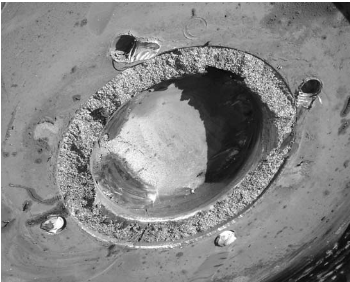
Figure 7 – Example of a Pulley with a Failed Shaft..
