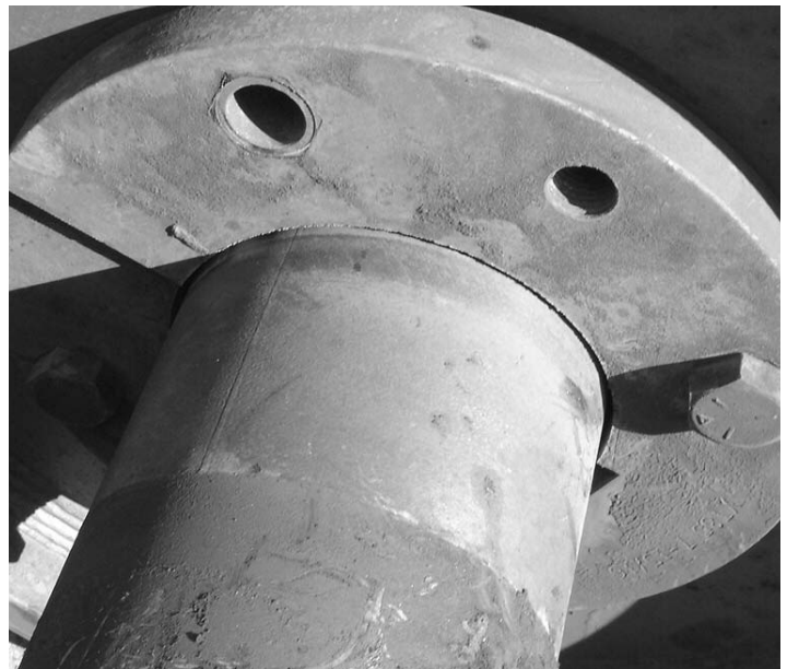
Figure 6 – Example of a Bushing that has been “wallowed”.
