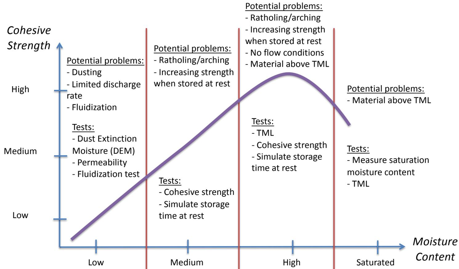
Note: Wall friction should be measured at all operating conditions as the friction of the material is independent of cohesive strength i.e. dry ore could have higher friction than wet ore.
