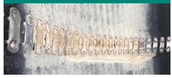
Mine in the southeastern US implemented Flexco Elevate™ and detected abnormal events with chatter events, which led to an investigation of the system. A failing splice was determined to be the cause as well as a poorly tensioned cleaner, respectively. Ultimately, the savings from a potential dropped belt were in the tens of thousands with significant downtime.
