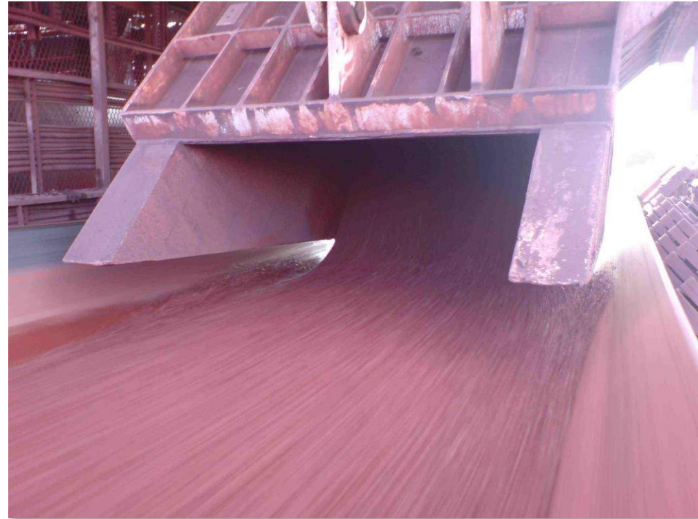
Proper belt loading with spoon
