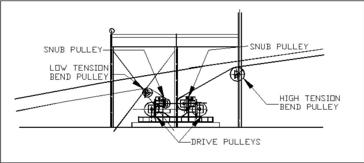
**Figure 3. Preliminary Design Drive Arrangement**
