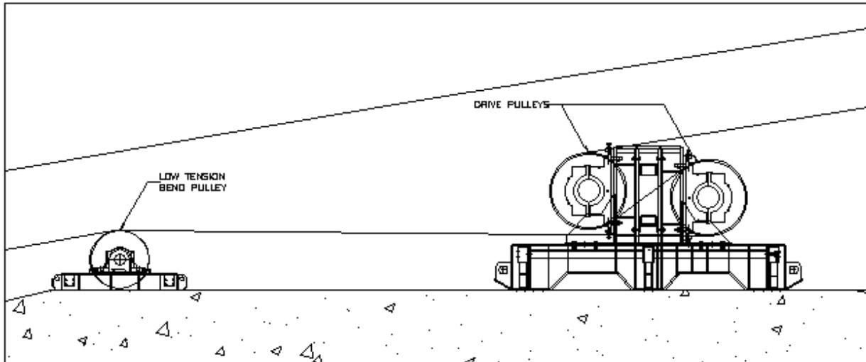
**Figure 7. Caterpillar Proposed Two Pulley Drive Layout**
