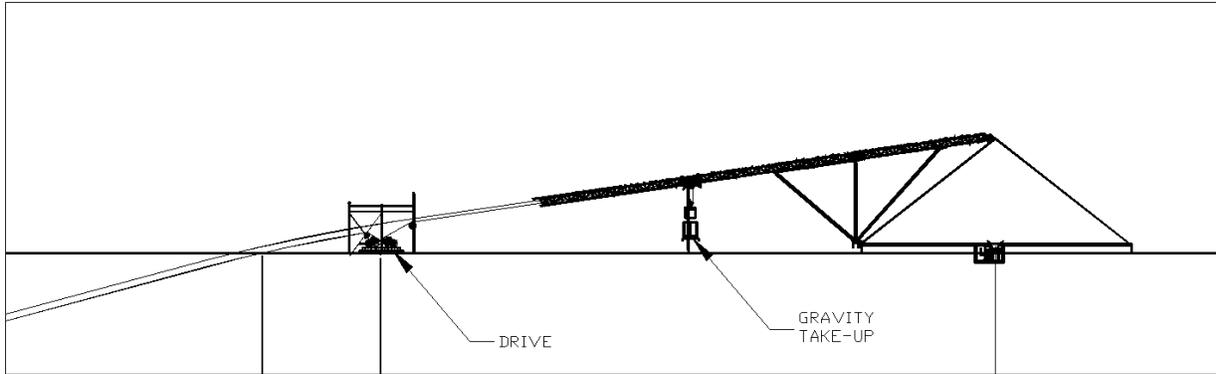
**Figure 2. Initial Location for Gravity Take Up**
