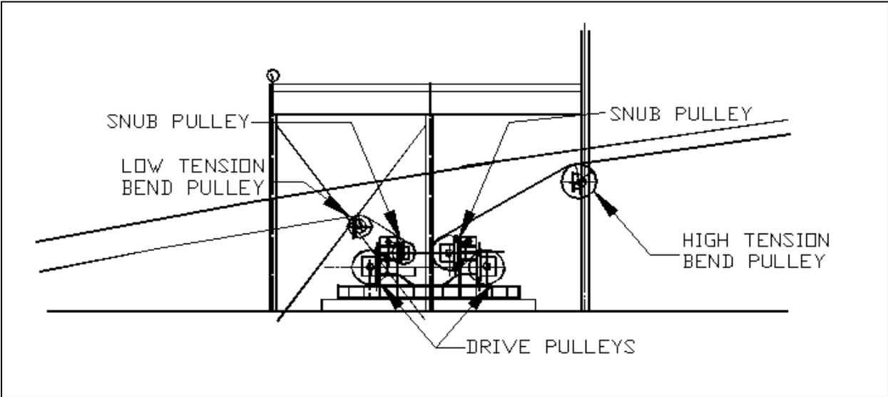
**Figure 3. Preliminary Design Drive Arrangement**
