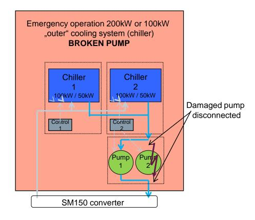
In case of a broken cooling pump it is possible to run the winder with one pump and full cooling capacity at normal operation
