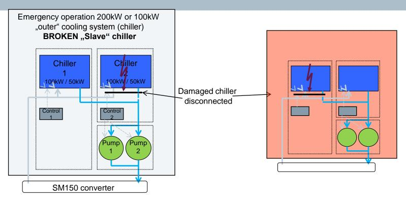
In case of a broken chiller it is possible to run the winder at 50% cooling capacity. The broken chiller will be disconnected and can be repaired.
